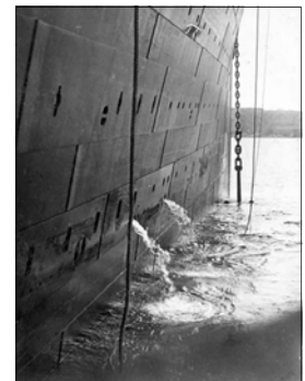
It took several minutes for the anchor to come to the surface. Titanic used six cables, 15 fathoms each, of wrought iron chain for its anchor. Image courtesy of TitanicPhotographs.com.
