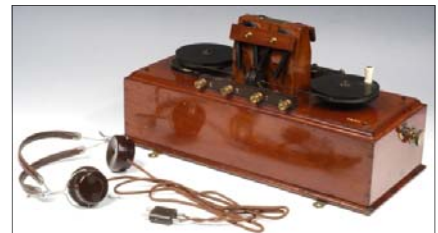
Marconi magnetic detector that received spark telegraphic signals in ships and shore stations. Image courtesy of mhs.ox.ac.uk .
